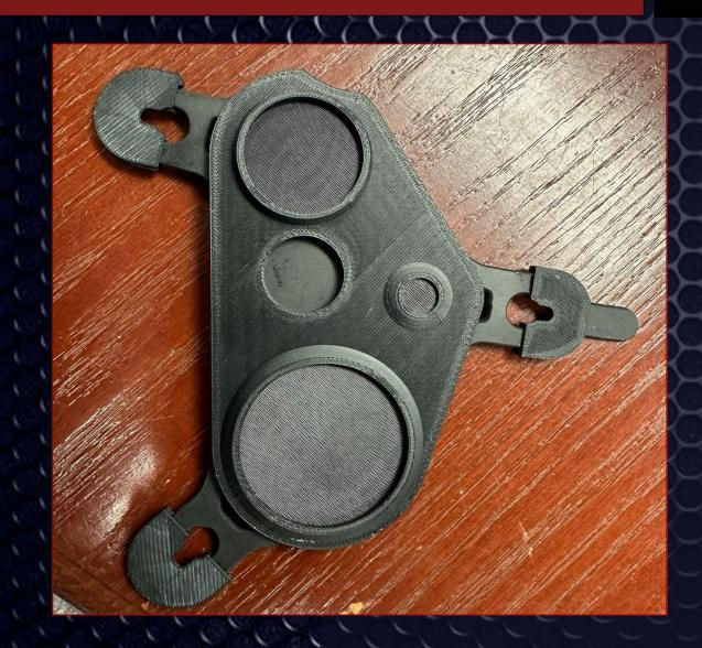
MDMC was asked by PM-FIRES to redesign the Lens Cover for the (Common Laser Range Finder-Integrated Capability (CLRF-IC) range finder. The rubber tabs were breaking off after use and due to the high cost (\$2,700.00) and low availability the range finders were dead lined. MDMC was able to redesign a 3D printed polymer replacement that was repairable, at a cost of (\$197.00). MDMC and PM-FIRES were able to increase readiness of CLRF-IC range finder in the FMF (Fleet Marine Force).
