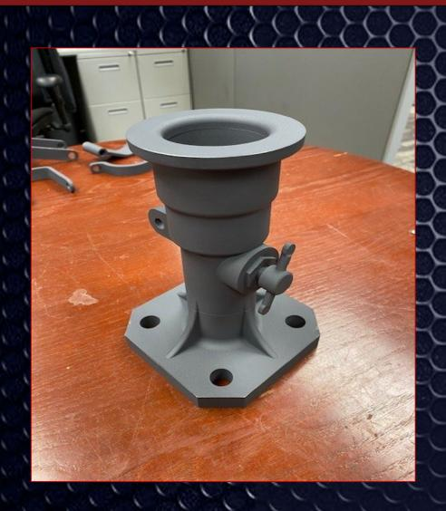
1<sup>st</sup> Recon Rigid-Hulled Inflatable Boat program suffering low readiness due to part obsolescence. MDMC was able to print these part for the machine gun mount in only a few days to help with these boats'
