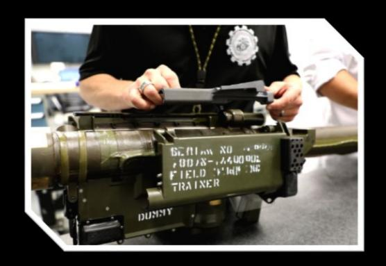
**Civilian-Marines from Marine Depot** Maintenance Command's (MDMC) Advanced Manufacturing Center of Excellence (AM COE) display 3D printed parts for use in the FIM-92 Stinger Missile System, while at Marine Corps Logistics Base Albany, Ga., April 20. MDMC manufactured the replacement parts in support of the Presidential Drawdown of security assistance, producing the parts in less than 24 hours.
