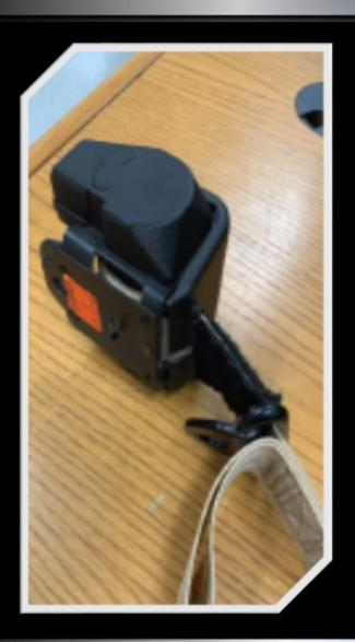
The dust cover for the Mine Resistant Ambush Protected Vehicle was a common failure item. The dust cover could not be purchased separately, MDMC was required to purchase the next higher assembly (entire seat belt assembly). Utilizing AM, MDMC was able to reverse engineer and 3D print the seat belt cover out of PC-ABS polymer, reducing the cost from \$920.00 to replace the entire seat belt assembly to \$14.77 to 3D print the dust cover.
