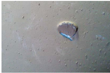
Figure 3 Serviceable (no fibers visible)
