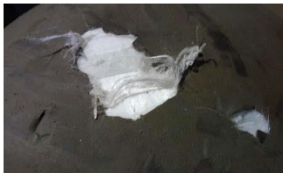
Figure 4 Unserviceable (fibers visible)
